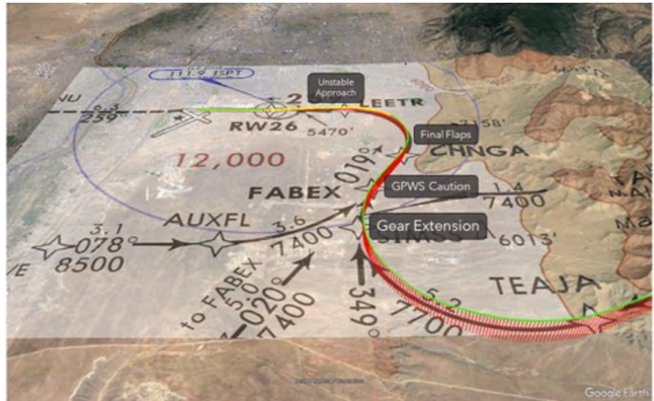
Figure 8: Google Earth image with overlaid approach plate, aircraft positions and data markers
