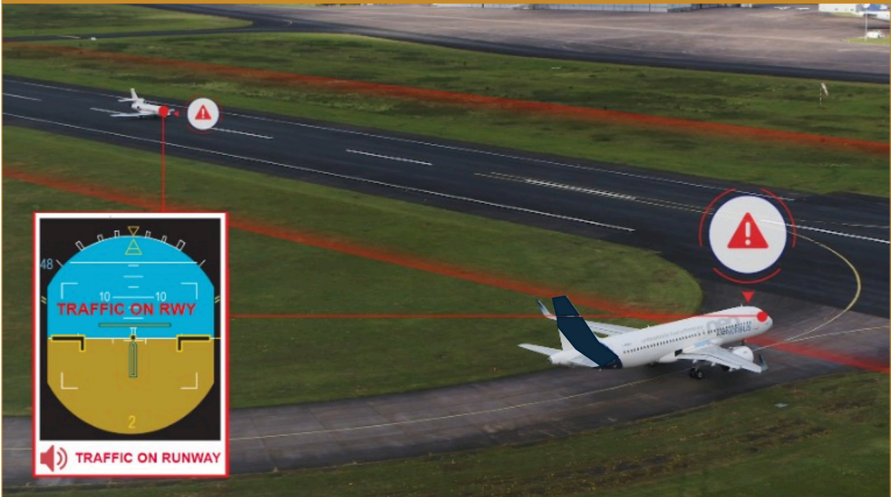
Figure 43. Example of SURF-A implementation showing a PFD - and the associated audio - alert (Airbus).
