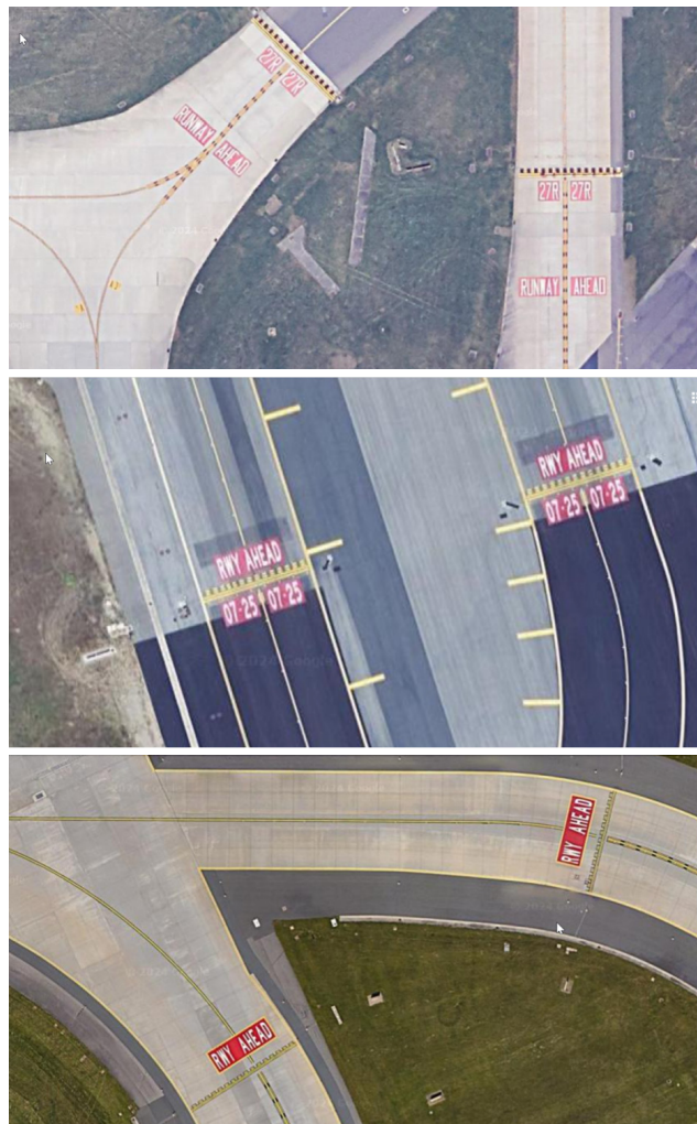
Figure 6. Example of 'RWY AHEAD' markings
