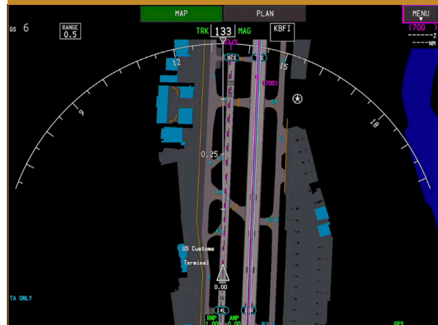
Figure 48. Example of aircraft on incorrect runway depicted on the navigation display (© Boeing)
