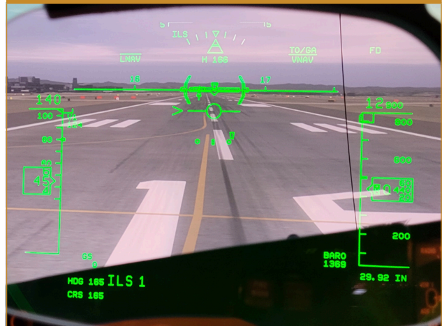
Figure 47b. Collins HUD on a Boeing 737 - line up on incorrect runway (© Boeing)
