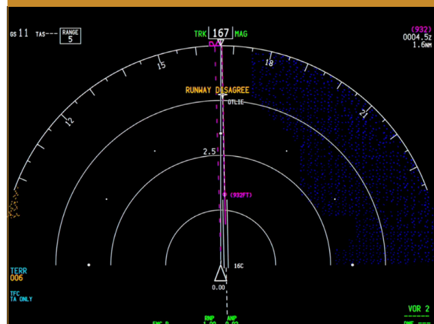
Figure 49. FMS runway disagree alert on the navigation display without airport map (© Boeing)
