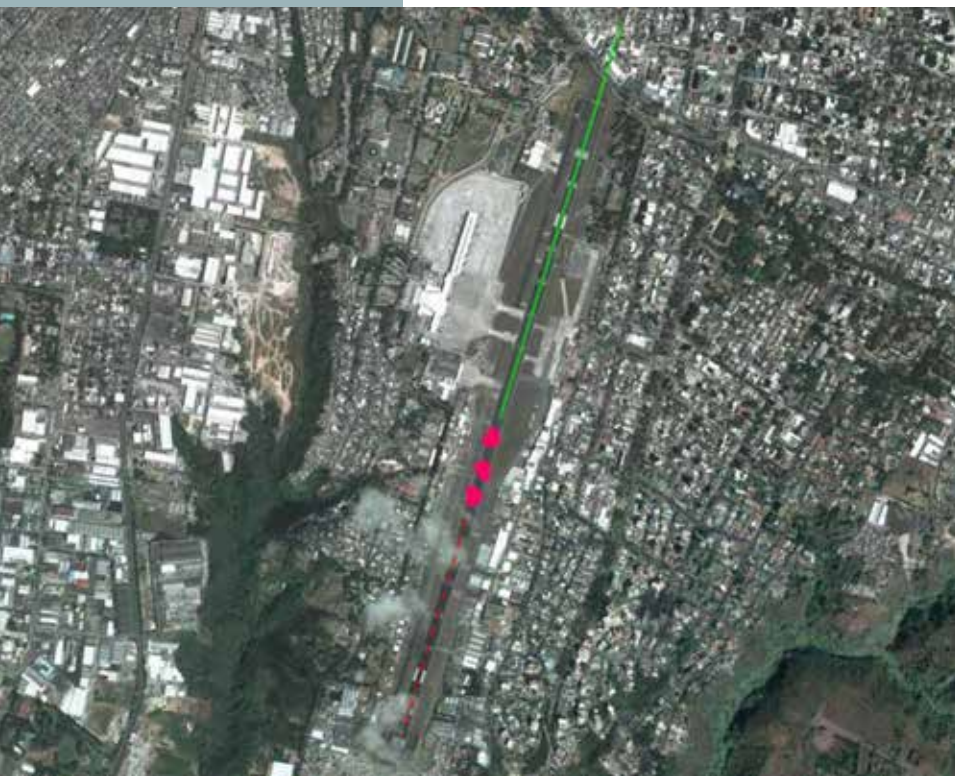
Satellite photo of Guatemala Airport. Magenta areas indicate positions where the on-board program recurrently indicated friction-limited braking. These positions were defined by the global positioning system, enabling comparison of multiple flights.
