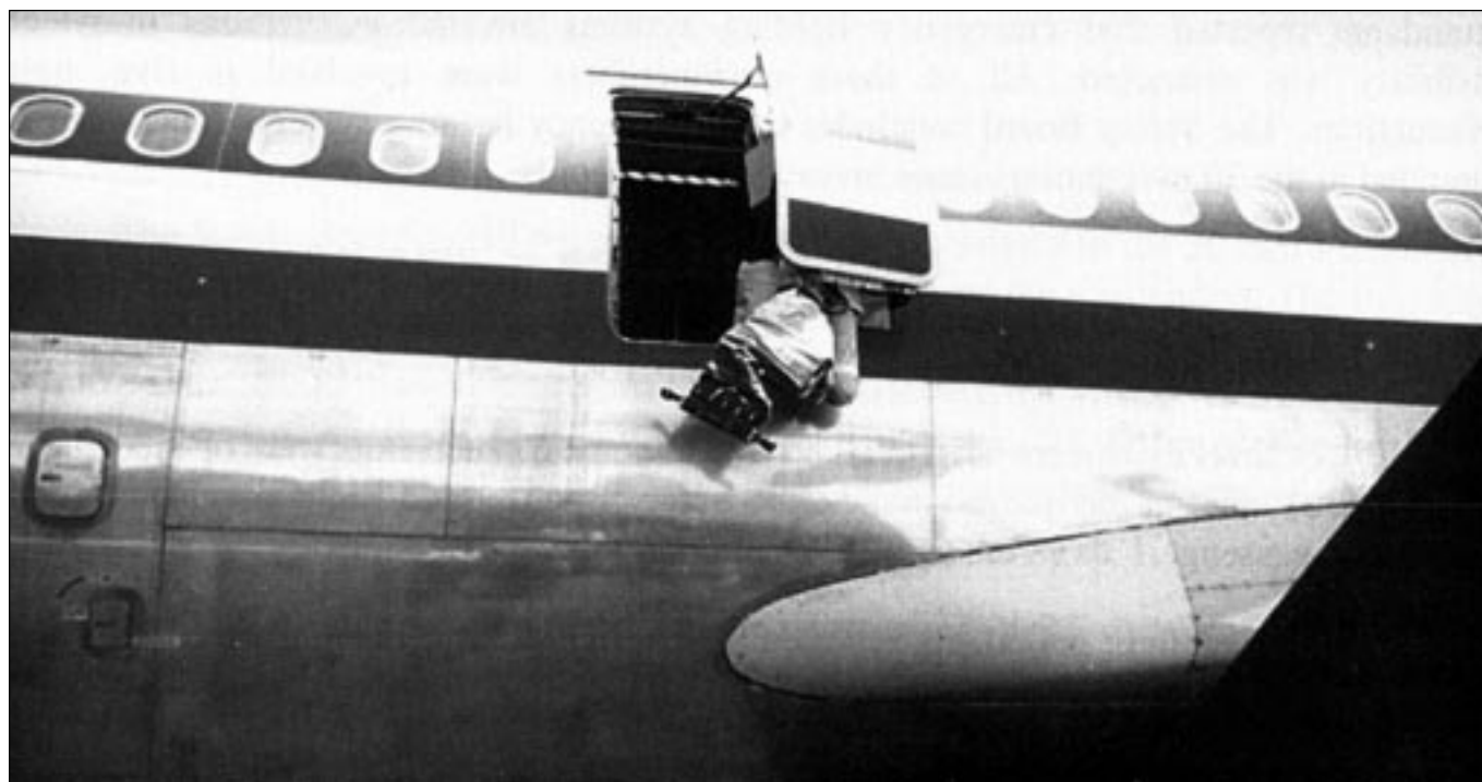
Figure 5-5. View of the R3 door that failed to operate as intended following the Airbus 300 accident on July 9, 1998, in San Juan, Puerto Rico (case 24).
