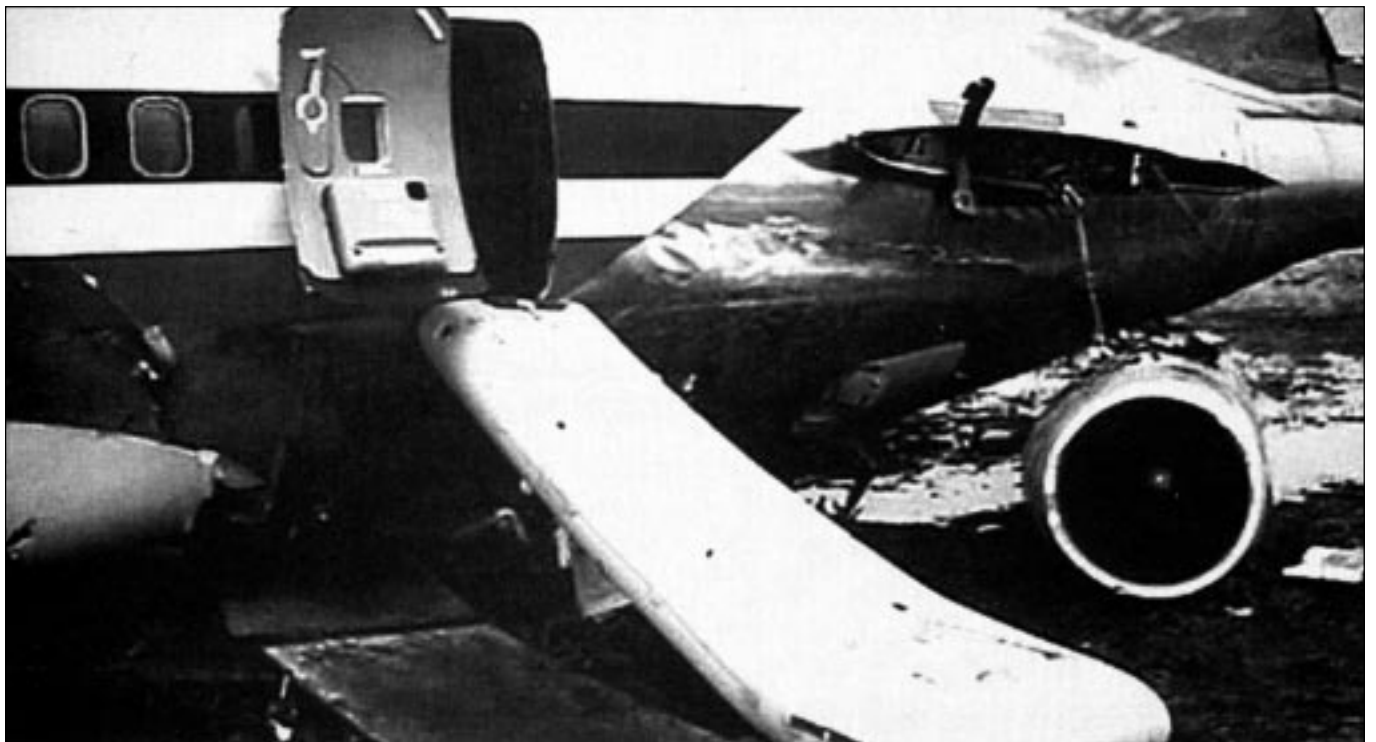
Figure 5-4. View of a slide used in the Boeing 727 evacuation on February 9, 1998, Chicago, Illinois (case 9).
