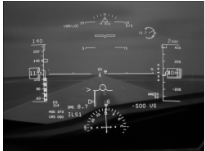
The dial symbol in the upper right corner of the display shows that angle-of-attack is 11.7 degrees. (Rockwell Collins Flight Dynamics)
