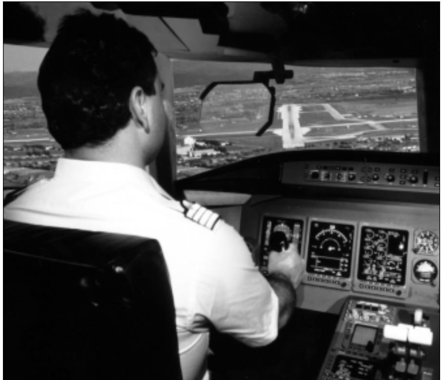
The combiner is relatively unobtrusive in the cockpit, visible here with a black frame on two sides between the pilot’s eyes and the runway. (Thales Avionics photo by Patrick Darphin)
