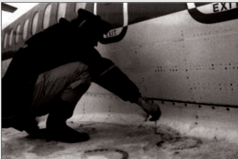
The tuft of parachute cord moved freely, but underneath the snow, clear ice had formed, and the cord's base was frozen solid.
