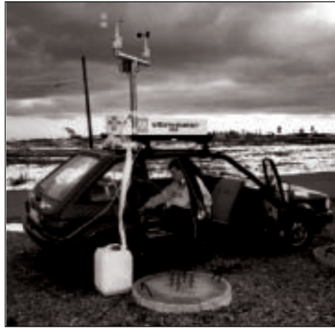
A car is equipped with a simulated aircraft aluminum fuel tank on its roof that has a Vibro-Meter electrical ice sensor built into the tank's upper surface. Various data, including wind speed, ambient temperature, fuel temperature and other information are recorded on a computer in the car. Several Finnair first officers conduct tests to determine optimum operating characteristics and standards for the sensor.
