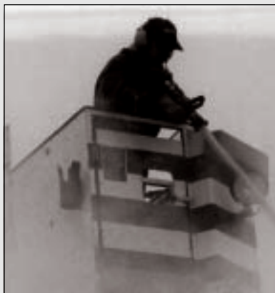
Hot water under high pressure in a tight stream was required to break ice free from an aircraft wing.
