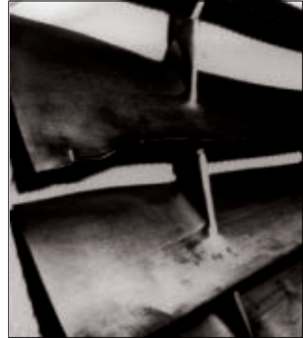
The gentle bend in the blades is characteristic of soft foreign object damage.
