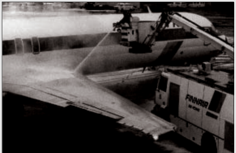
Ice forms more readily over the wing root, where the cold fuel settles and there is more metal structure, including the landing gear components, which can contribute to colder temperatures.
