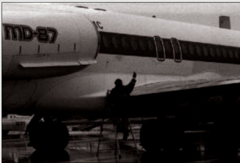
The mechanic gave a "thumbs-up" acknowledgment to the deicing truck crew that the wing surface was clean and there was no ice on it.
