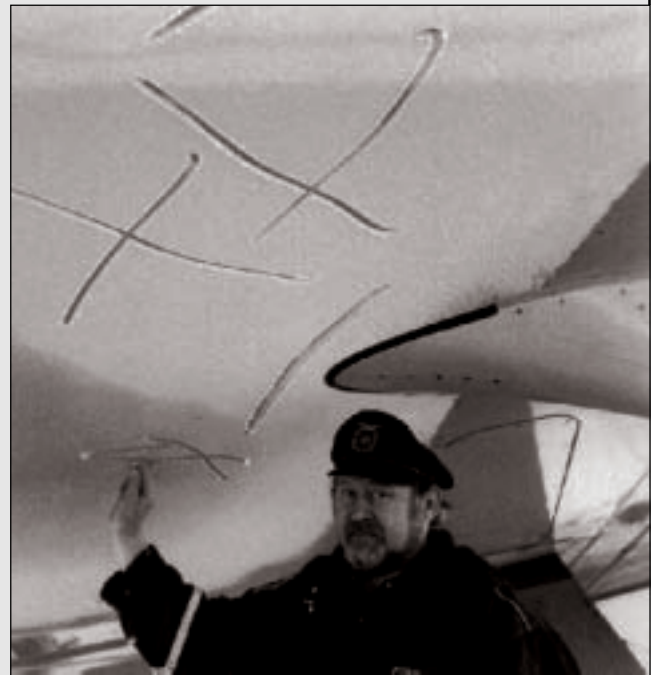
Frost formed readily under the wings in the fuel tank area.
