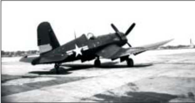
An F-4U equipped with an auxiliary rudder was one of the first variable-stability research aircraft.
