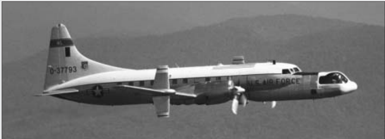
Front cockpit of total in-flight simulator (TIFS) airplane recently was used to test synthetic-vision systems.
