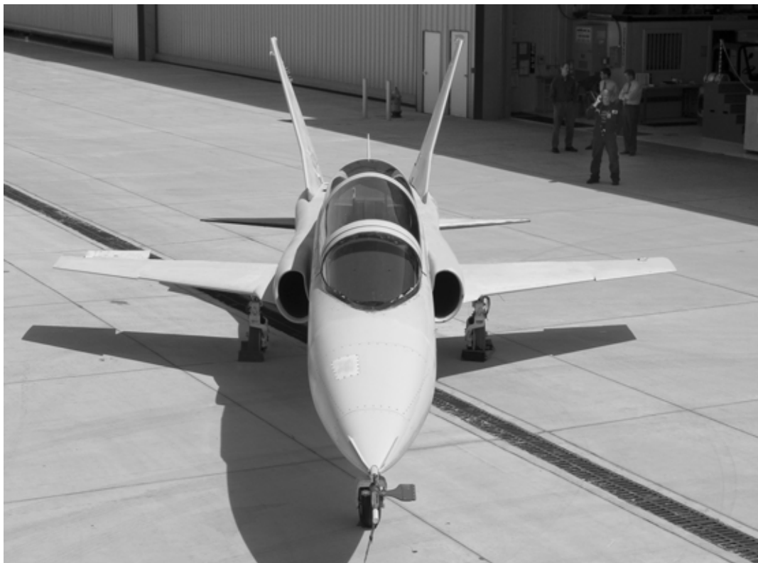
Near-Mach 1 speed and structural limits of +6 g and -3 g are planned for the Javelin, which has two engines, two seats and dual controls. (Photo: Aviation Technology Group)
