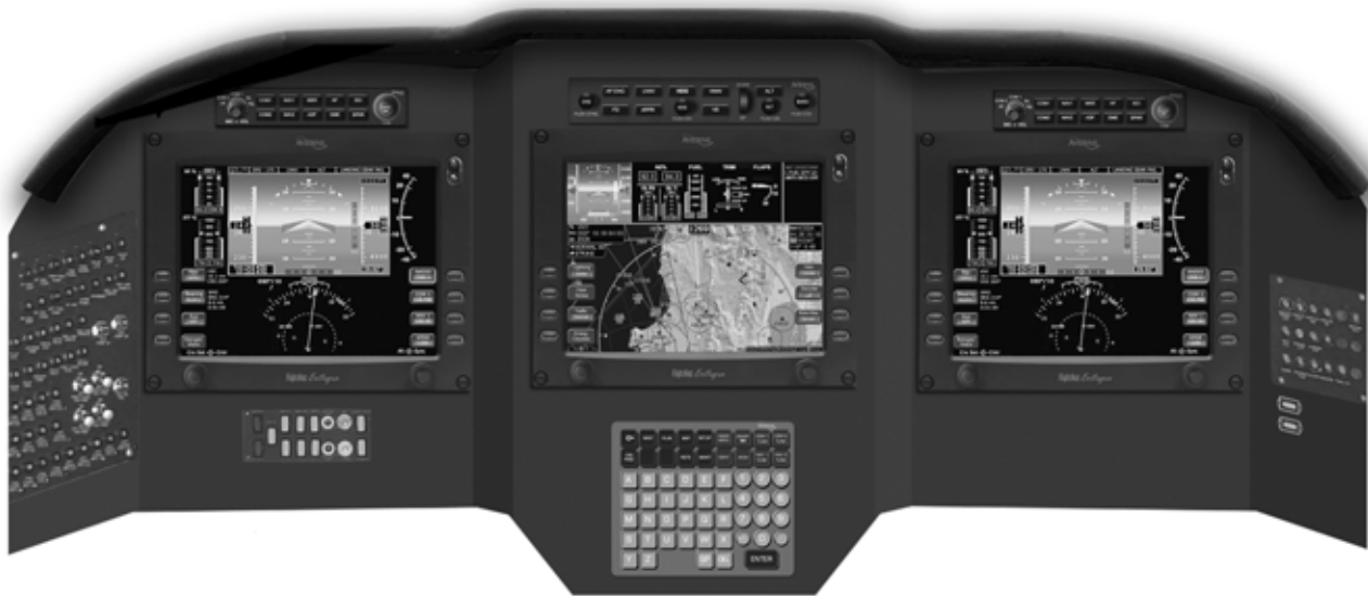
A mock-up of an Avidyne FlightMax Entegra panel planned for the Adam Aircraft A700 shows three flat-panel, liquid-crystal displays. (Photo: Avidyne Corp.)
