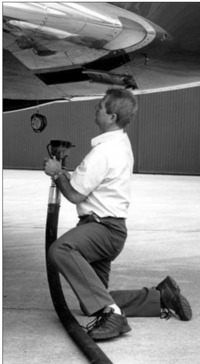
FSF auditors look for supervision and control of aircraft servicing by pilots or maintenance personnel. Here, maintenance technician Steve Ogden prepares to fuel a Gulfstream IV. (FSF photo)
