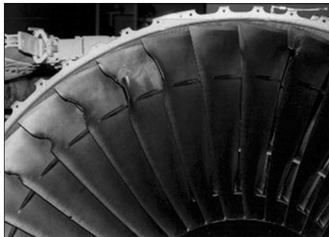
Fan blades bent by ingestion of a bird. Photo: U.S. Federal Aviation Administration
