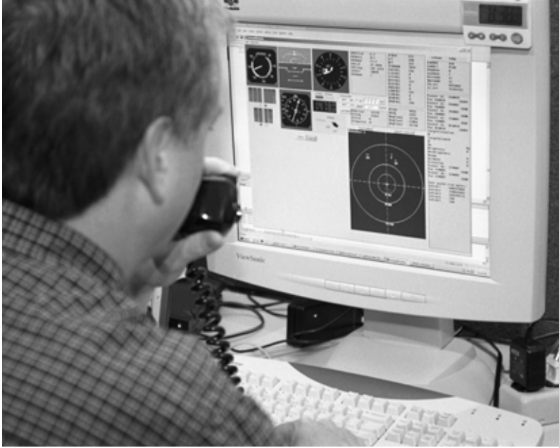
A ground-based pilot flies the Scaled Composites Proteus aircraft during collision-avoidance testing by NASA. (Photo: Tom Tschida, NASA)
