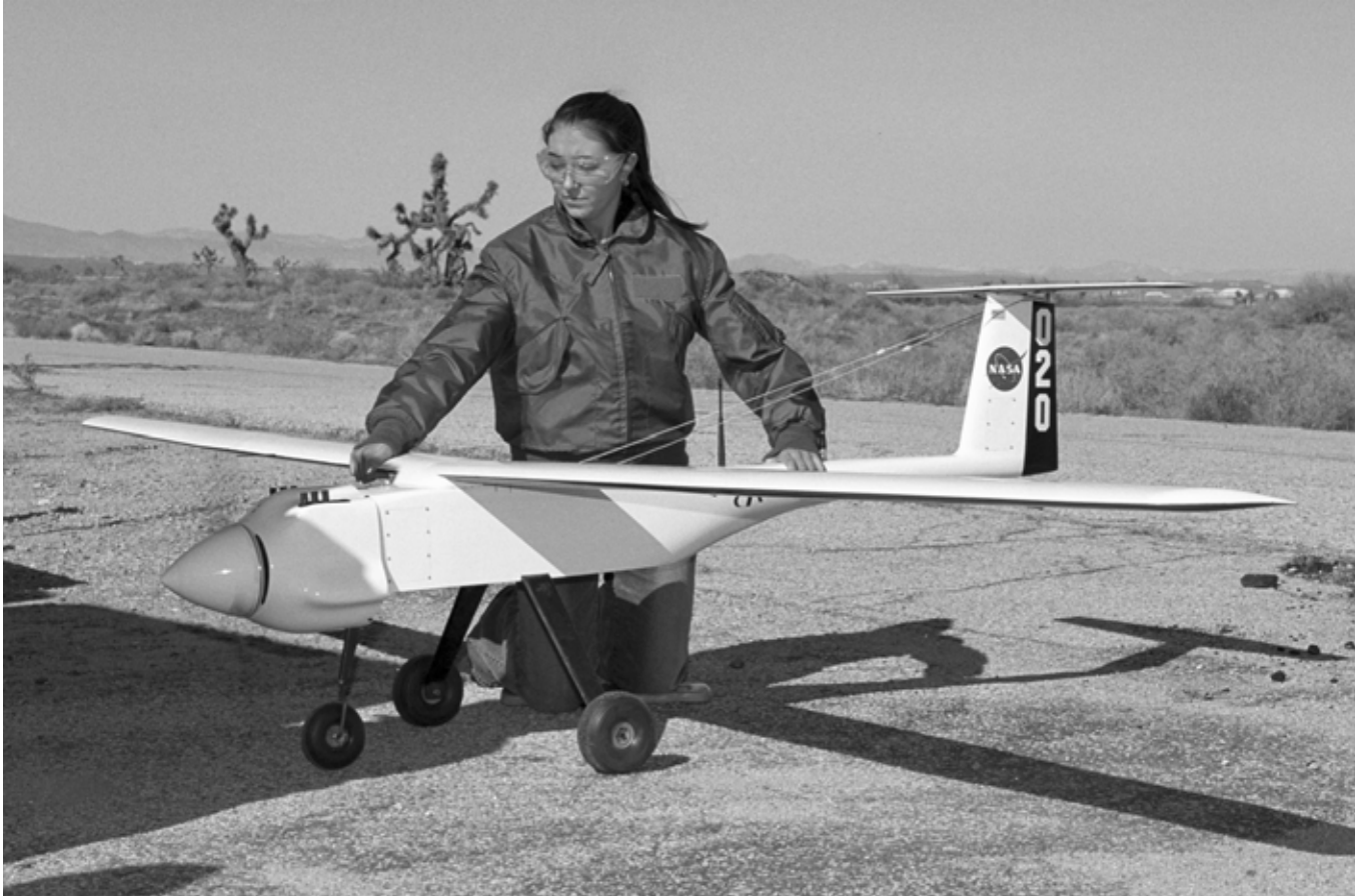
The RnR Products APV-3 has an eight-hour endurance at 45 knots and a maximum cruise airspeed of 90 knots. Shannon Kolensky, a cooperative-program student, holds the aircraft during engine runup. (Photo: Tom Tschida, NASA)
