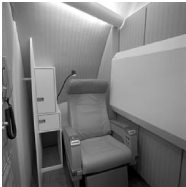
The flight crew-rest facility in the Airbus A340-500 provides reclining seats when the bunks are stowed.
