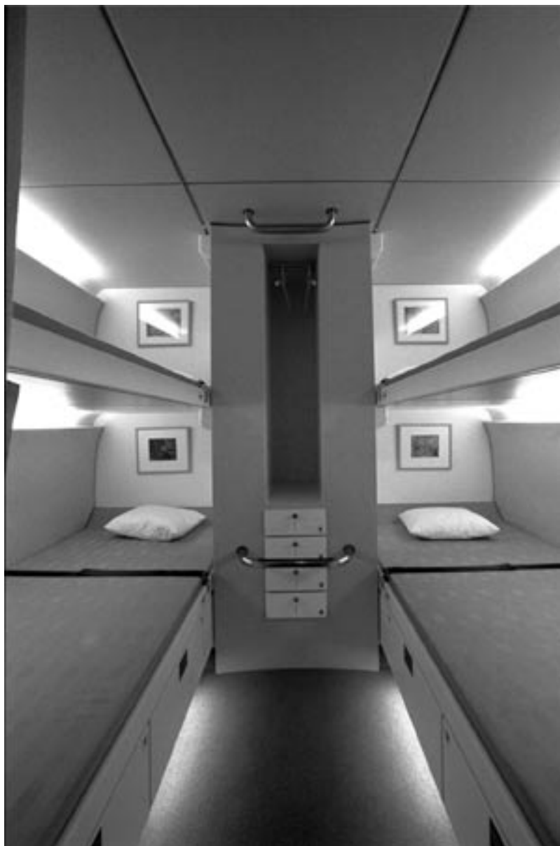
Crew-rest facility for Airbus A340-500 cabin crewmembers.
