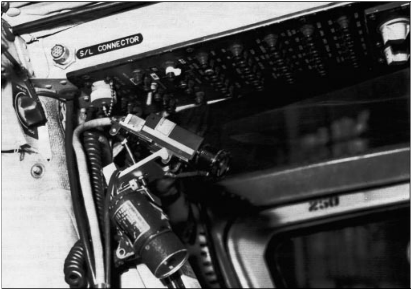
To record crew tasks, a miniature tv camera was mounted at the base of the overhead panel at the rear of the cockpit, where it could "look" over the pilots' shoulders while they performed flying tasks.
