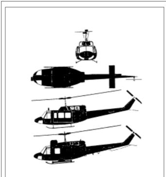
The Bell model 212 twin-turboshaft helicopter first flew in 1968. Production of the 15-seat utility helicopter was transferred to Canada in 1988. The Bell 212 is powered by a Pratt & Whitney Canada PT6T-3B Turbo Twin Pac, comprising two PT6 turboshafts. It has a maximum range of 227 nautical miles (420 kilometers).
