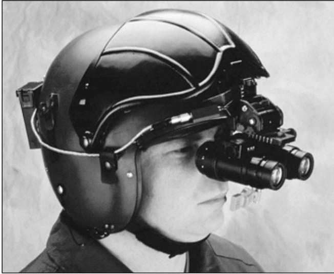
Night vision goggles use image intensification tubes to amplify existing light to allow the human eye to see more easily in darkness. (Photo: Aviation Specialties Unlimited)
