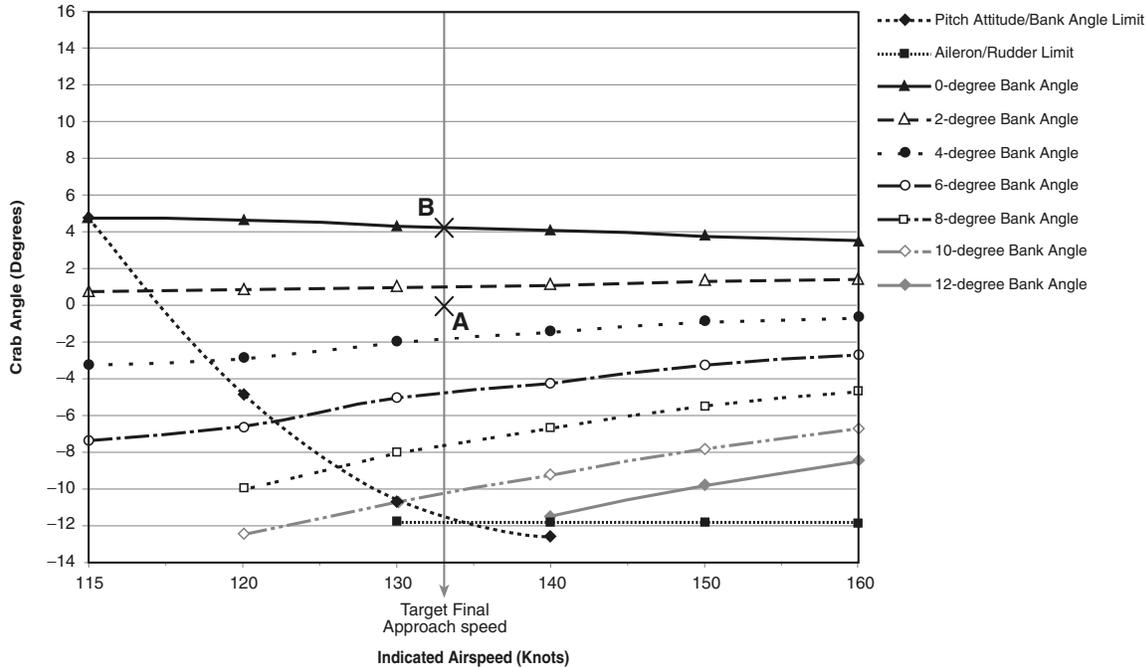
Examples: A sideslip landing (zero crab angle) requires about a three-degree bank angle at touchdown (point A). A wings-level landing (no decrab) requires a crab angle between four degrees and five degrees at touchdown (point B).
