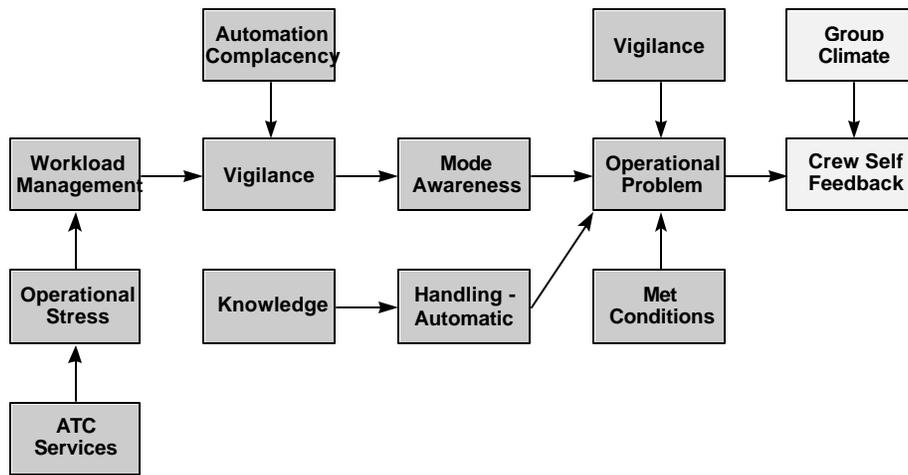
Figure 5 Event Sequence Diagram – Overspeed in Descent
