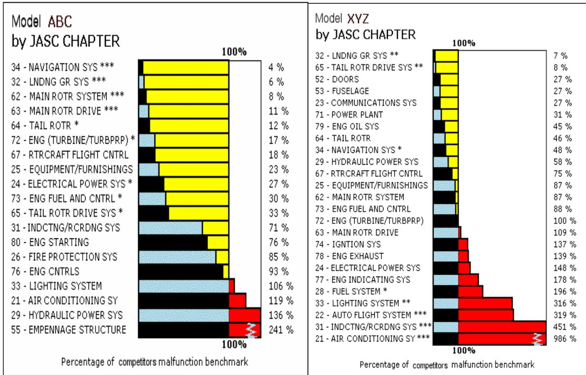
**Figure 4 Two Different Models Showing Malfunction Ratios by Mechanical System**
