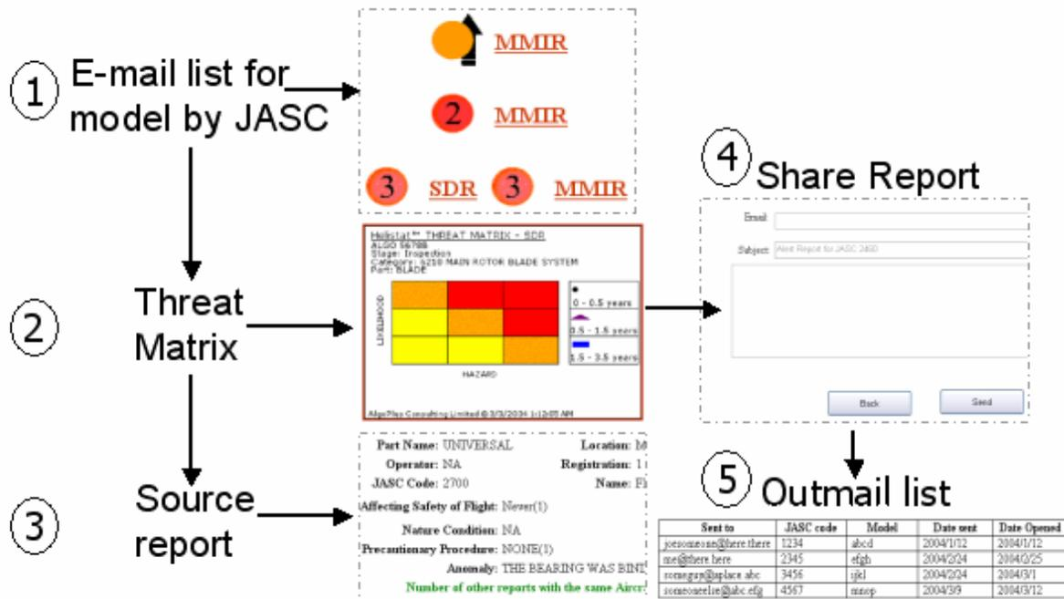
Figure 1 Elements of the JetStat System
