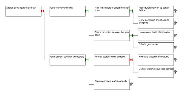
Figure 4 Dependency Model – Landing Gear
