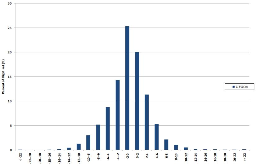
Airspeed (Calibrated) Minus Vapp at Estimated Threshold Crossing (knots)
