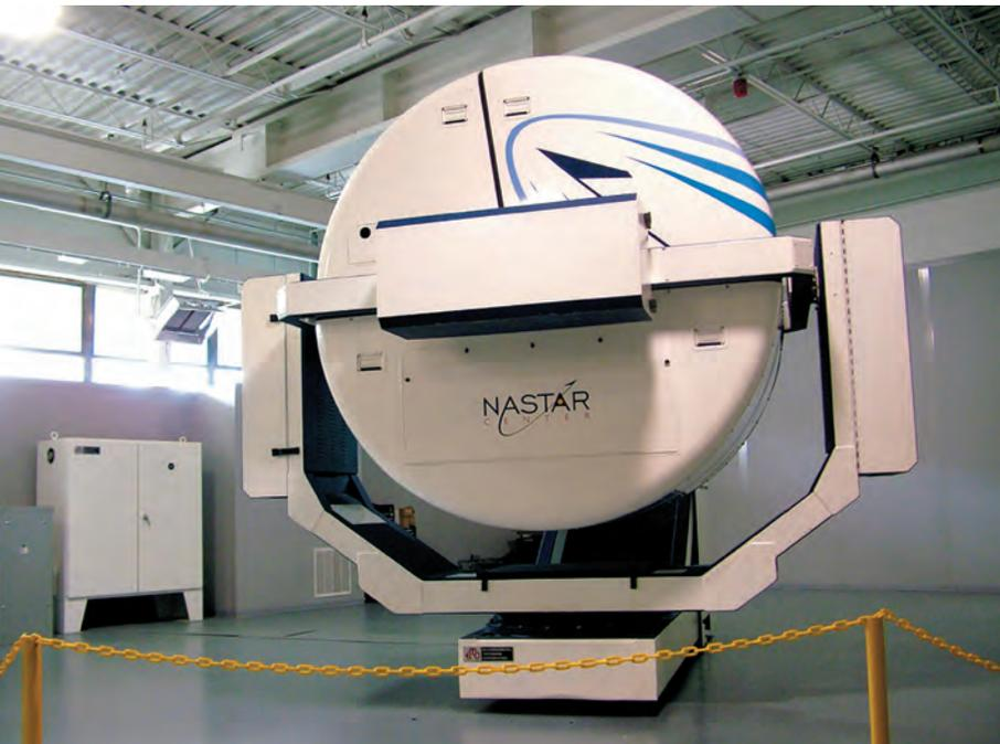
The single-seat Gyrolab GL-2000 provides controlled, sustained g-force with its planetary axis, and provides 360-degree rotation in yaw, pitch and roll axes.
