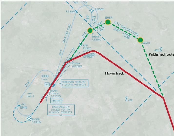
**Notes:** The aircraft intercepted the localizer inside the final approach fix and about 1,000 ft above the 3-degree glideslope.
