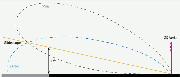
**Notes:** The null between the 90Hz (fly-down) and the 150 Hz (fly-up) signals defines the 3-degree glide path.
