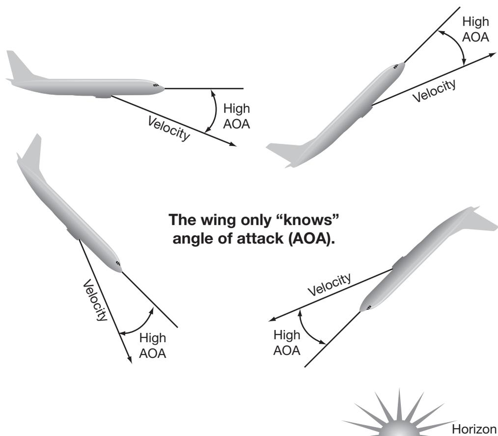
should not expect the airplane to remain unstalled just because the indicated airspeed is higher than AFM chart speeds, because the conditions may be different.
