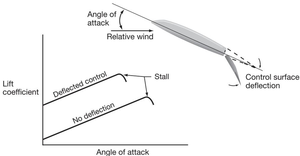
be unstalled in order for the aerodynamic controls to be effective.
