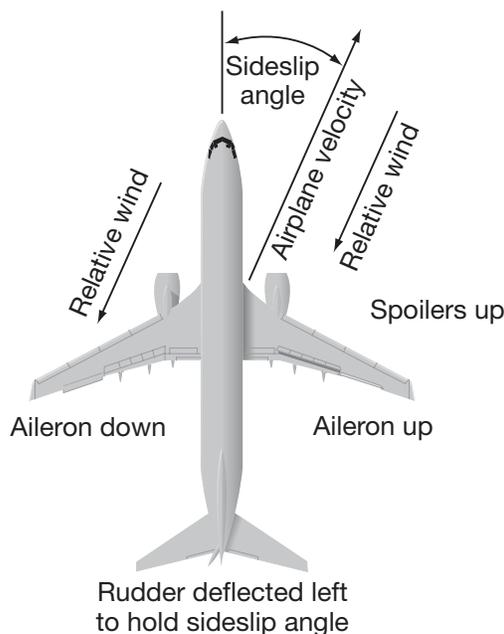
With the exception of crosswind landing considerations requiring pilot-commanded sideslip, commercial transport airplanes are typically flown at or very near zero sideslip. This usually results in the lowest cruise drag and is most comfortable for passengers, as the sideways forces are minimized.
