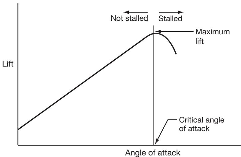
Instead of increasing with an increase in angle of attack, it decreases. At this critical angle of attack, the air moving over the upper surface can no longer remain attached to the surface, the flow breaks down, and the surface is considered stalled.
