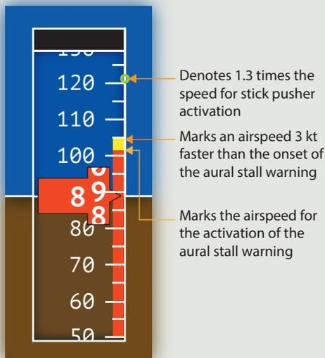
**Notes:** The top display shows stall-warning indications similar to what the accident pilot saw. The bottom display shows indications appropriate for icing conditions, which would have been presented if the ice-protection system had been activated.
