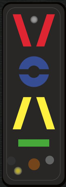
An example of an AOA indicator (Icon A5 Angle of Attack Safety System, p. 29) and an example of an AOA indexer (Alpha Systems AOA Griffin, above) — each FAA-approved strictly for pilots' supplemental reference and only in GA aircraft — have similarities to their standard counterparts in military jets and to their optional counterparts in large commercial jets and business jets.
