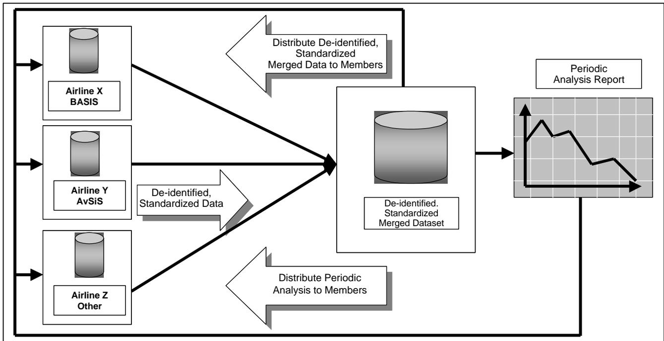
Figure 2-Periodic Aggregation and Analysis System Functional Diagram
