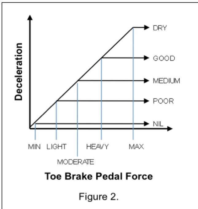
In addition, some aircraft manufacturers provide advisory landing distance performance information as a function of pilot braking action reports. They do this by choosing a conservative aircraft braking coefficient for the braking action terms of good, medium and poor. The appropriate value of aircraft braking coefficient is used in the manufacturer's advisory landing distance calculations.
