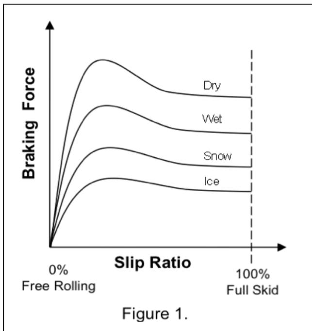
imum slip ratio regardless of the surface conditions. The optimum slip ratio can be thought of as the anti-skid limit. The pilot has control of the level of wheel slip through the application of pedal braking as long as the anti-skid limit is not reached. Once the anti-skid limit is reached, pressing the brake pedals any harder will not increase the wheel braking force because the runway friction capability has been reached.
