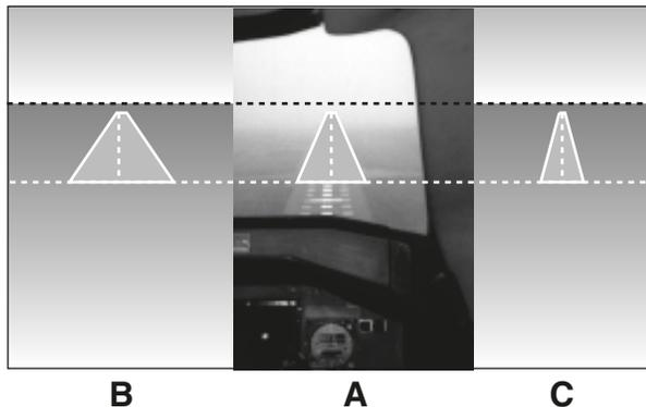
Note: All three panels show a pilot's sight picture from an aircraft at 200 feet and on a three-degree glide path. The runway in panel A is 150 feet (45 meters) wide and 11,500 feet (3,500 meters) long. The runway in panel B is wider/shorter than the runway in panel A; the crew may believe that the aircraft is on shallower-than-actual glide path. The runway in panel C is narrower/longer than the runway in panel A; the crew may believe that the aircraft is on steeper-than-actual flight path.
