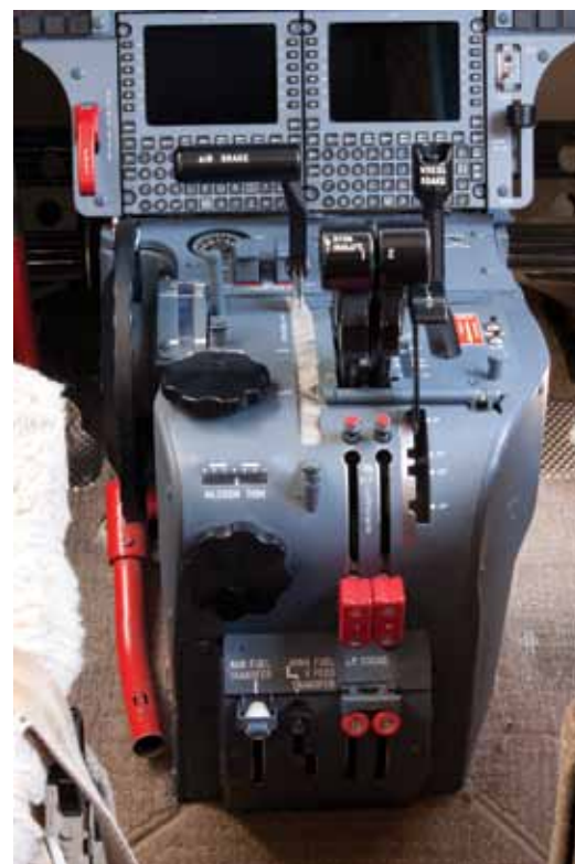
The captain pulled the 'AIR BRAKE' handle all the way back, to engage the lift-dump system, nine seconds after touchdown.
