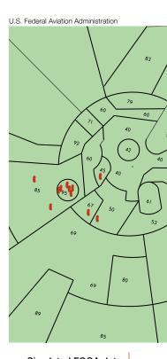
Simulated FOQA data, overlaid in red on an illustration of an ATC radar display, show that a sector with a minimum vectoring altitude of 9,500 ft, marked as "95," had the most TAWS alerts on the day studied.
