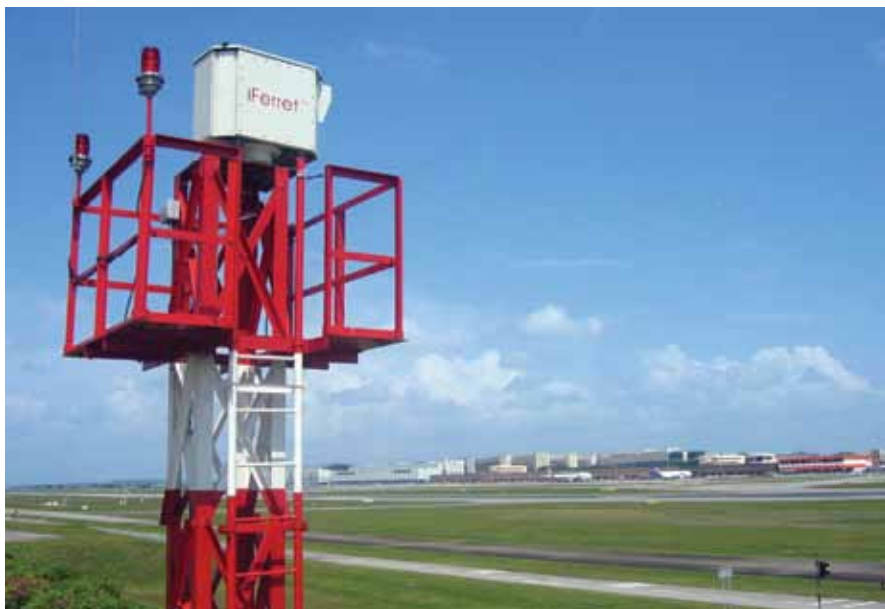
Stratech Systems' iFerret is an electro-optical system that can be used to monitor taxiways and aprons, as well as runways, for FOD.
