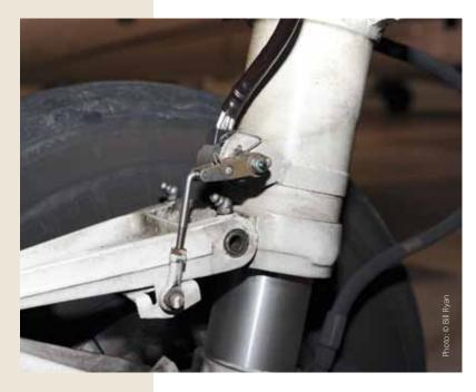
An incorrectly adjusted squat switch prevented the cabin from pressurizing when the landing gear was retracted. the figure, but it apparently was low enough to cause the pilot to perceive that the aircraft had a 100-kt head wind. (The aircraft actually had a slight tail wind.)
