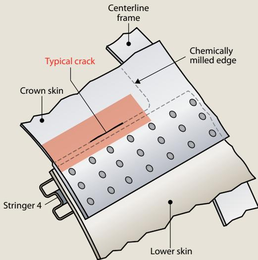
Note: Cracks were found above the left forward passenger door.
