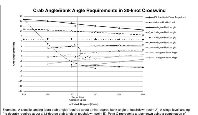
(no decrab) requires about a 13-degree crab angle at touchdown (point B). Point C represents a touchdown using a combination of sideslip and crab angle (about five degrees of bank angle and about five degrees of crab angle). Point D represents a steady-sideslip landing conducted about four knots above  $V_{\text{REF}}$ .
