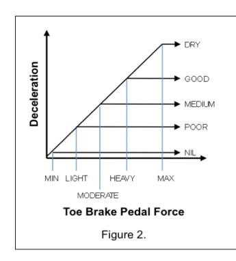
In addition, some aircraft manufacturers provide advisory landing distance performance information as a function of pilot braking action reports. They do this by choosing a conservative aircraft braking coefficient for the braking action terms of good, medium and poor. The appropriate value of aircraft braking coefficient is used in the manufacturer's advisory landing distance calculations.
