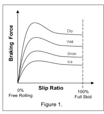
mum slip ratio regardless of the surface conditions. The optimum slip ratio can be thought of as the anti-skid limit. The pilot has control of the level of wheel slip through the application of pedal braking as long as the anti-skid limit is not reached. Once the anti-skid limit is reached, pressing the brake pedals any harder will not increase the wheel braking force because the runway friction capability has been reached.
