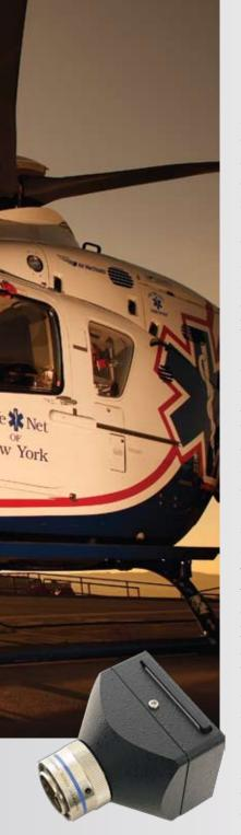
Quick access recorders, like the one pictured here, are being installed in Air Methods helicopters as part of a FOQA data development project. Safety Foundation has been among them, with the release in 2009 of the *Industry Risk Profile* developed by Aerosafe Risk Management, which criticized the widely varying standards and conflicting practices throughout the industry.<sup>3</sup>
