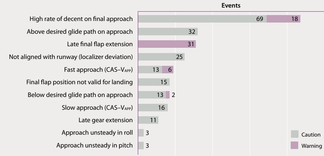
C-FOQA = corporate flight operational quality assurance; CAS = calibrated airspeed; V<sub>APP</sub> = approach speed
