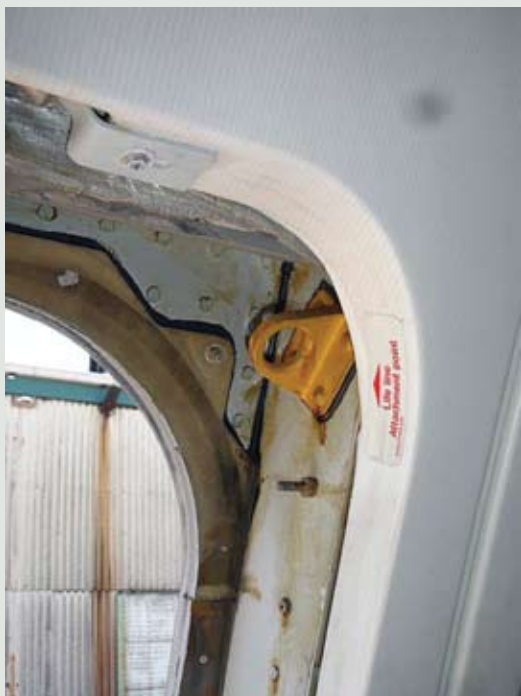
Top, one passenger jumped into the 41° F (5° C) Hudson River from door 1L before the slide/raft was deployed manually; bottom, overwing-exit life line-attachment points were unused, and nine passengers fell into the water.
