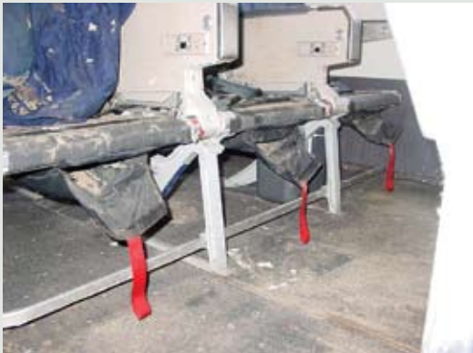
Top, life vest storage pouches were beneath economy-class seats on Flight 1549; bottom, the FAA had tested four underseat stowage configurations.
