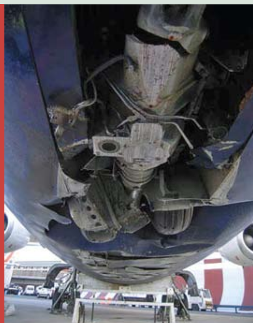
The Avro 146’s lower fuselage was damaged after the landing gear’s collapse. Above, the accident airplane, photographed on another day, at London City Airport.
