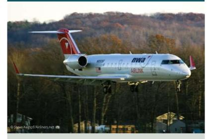
he first in Bombardier's line of Canadair Regional Jets, the CRJ100 began service in 1992 and shares the engineering designation CL600-2B19 with the Challenger business jet, on which its design was based. Increases in maximum takeoff weights and fuel capacities resulted in the extended-range (ER) and long-range (LR) versions.
