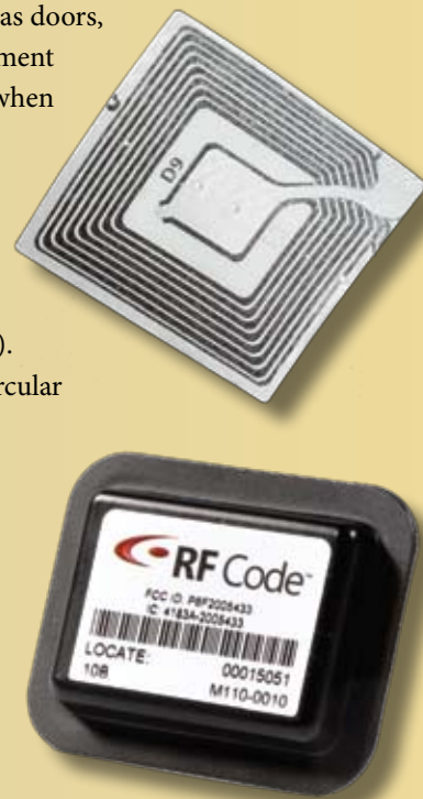
Radio frequency identification devices (RFIDs) include the passive RFID, top, and the low-power active RFID.
