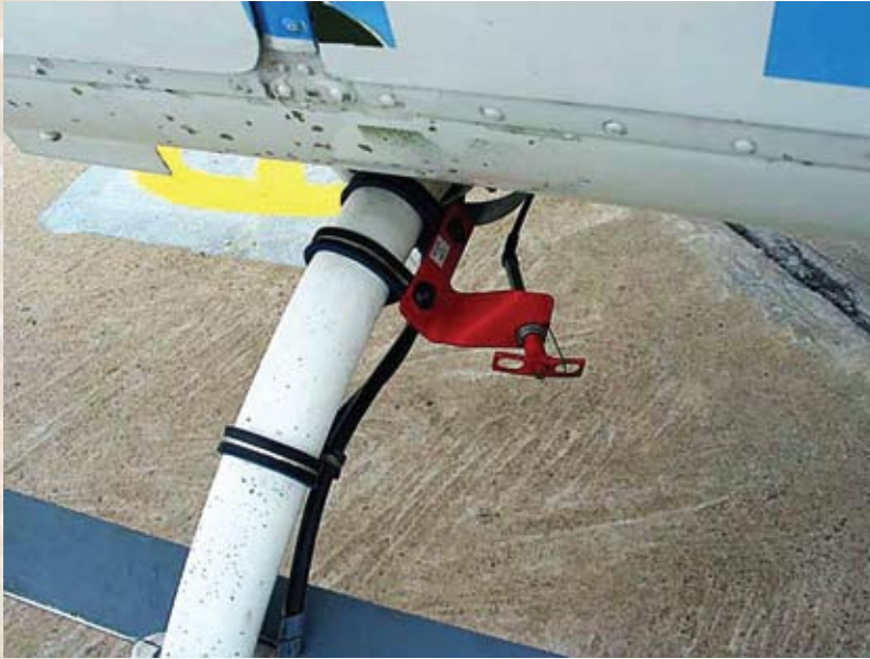
Life rafts on the Bell 206L1 could be activated from inside the helicopter or by pulling either of two red external T-handles.
