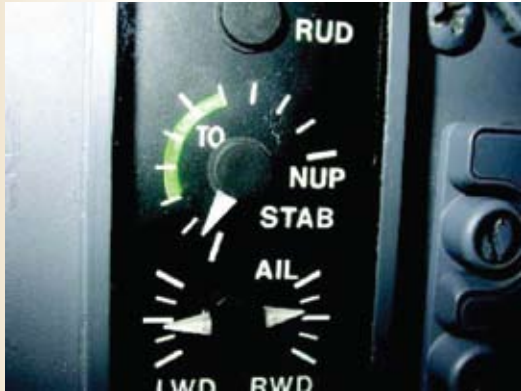
This Bombardier Challenger 600 pitch-trim position indicator is similar to one examined in the Teterboro crash.
