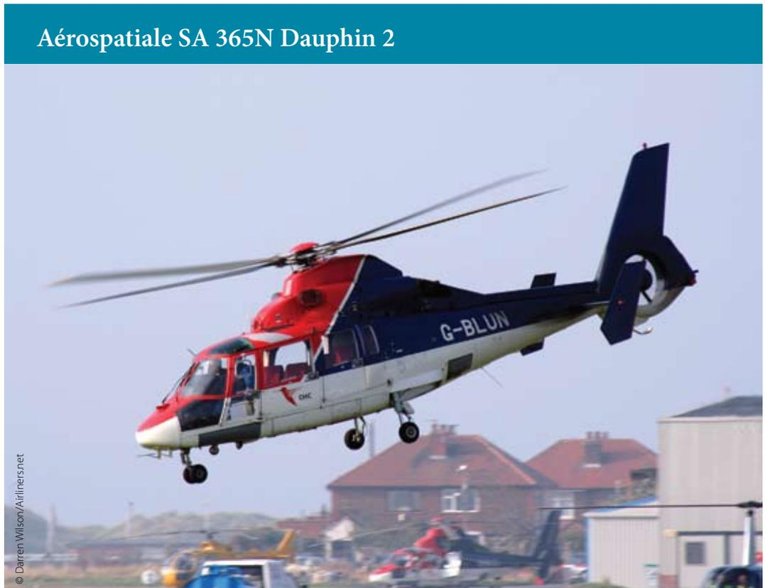
**T**he Aérospatiale (now Eurocopter) SA 365N, first flown in 1979, is a twin-engine helicopter designed to carry two pilots and up to eight passengers. It is equipped with Turbomeca Arriel 1C gas turbine engines, each rated at 530 kW (710 shp).
