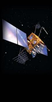
In March 2009, the U.S. Air Force tested transmission of the new L5 signal from a GPS block IIR-M satellite, illustrated above. Below, USAF Tech. Sgt. Randall Thomas, right, of the 1st Space Launch Squadron, monitors pre-launch mating of the actual satellite to the Delta II rocket.
