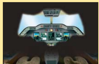
Uncontrolled smoke in the cockpit -Visibility with EVAS
