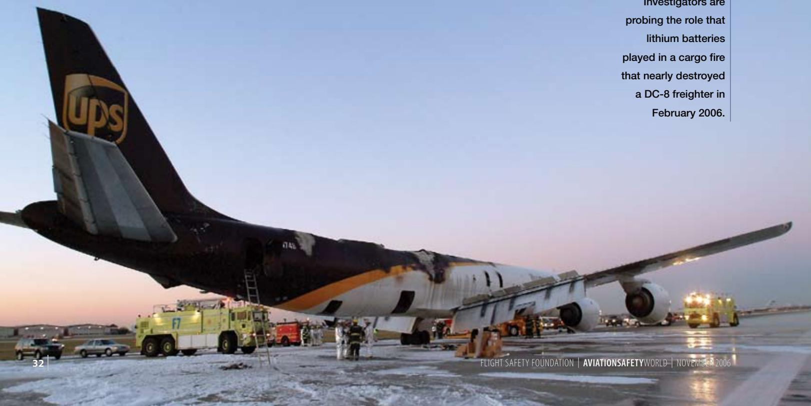
Investigators are probing the role that lithium batteries played in a cargo fire that nearly destroyed a DC-8 freighter in February 2006.
