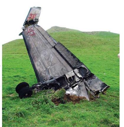
"The probable explanation for the bank angle excursion and the altitude loss is that the autopilot had disengaged automatically as a result of a servo reaching its torque limit," the report said. "With the autopilot constraint removed, the aircraft abruptly responded to the trimmed rudder input by rolling left and starting to yaw its nose down into a steeply banked diving attitude."
