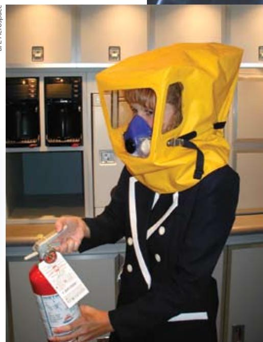
Clear polycarbonate visor panels in this PBE design provide a wide field of vision.
