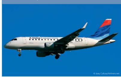
he ERJ-170, which first flew in 2002, has 70 to 80 passenger seats and is powered by General Electric CF34-8E5 engines. Standard maximum weights are 79,344 lb (35,990 kg) for takeoff and 72,311 lb (32,800 kg) for landing. Maximum range is 2,000 nm (3,704 km).
