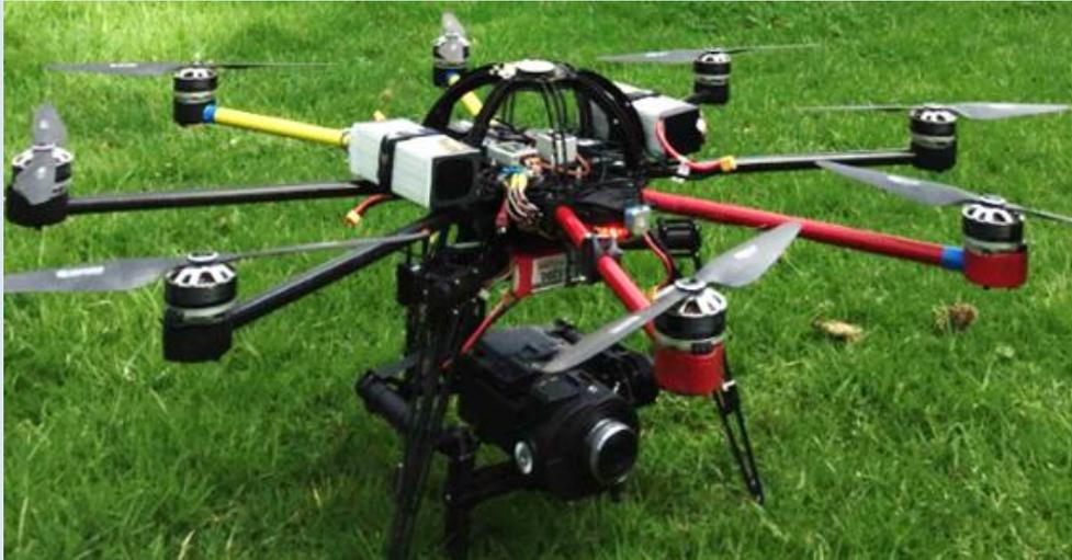
Aeronavics SkyJib 8 remotely piloted aircraft from AO-2015-035. Source: RPAS operator
