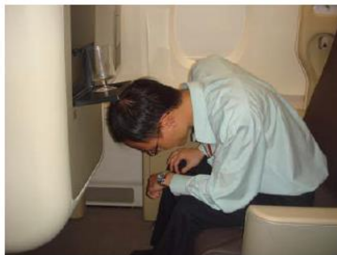
Cup holder fold up when hit from bottom
