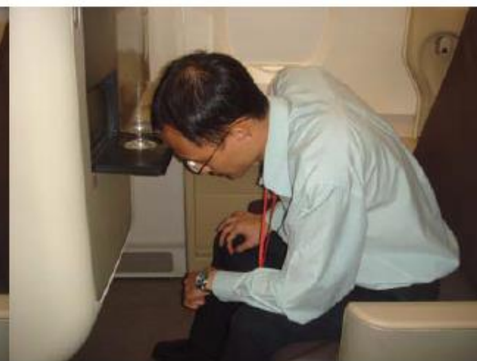
Cup holder would unhinge when hit from top
